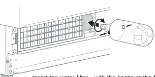
Insert the water filter - with the knobs at the front in a horizontal position - as far as it will go and turn clockwise until it snaps in. Touch
