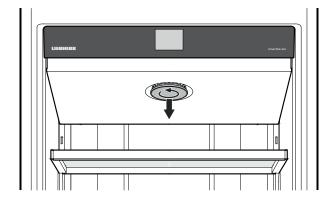
Turn the cover anticlockwise and remove it.
